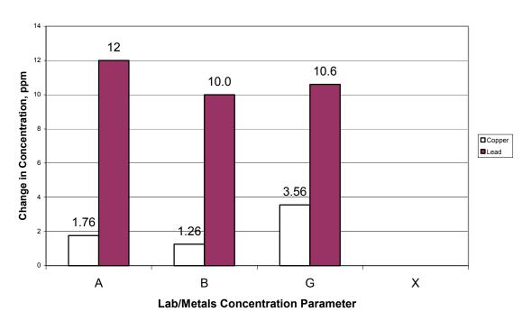
Precision estimates for Copper illustrate good agreement between labs A and B, while lab G shows higher variability. Precision estimates for Lead show reasonable agreement across all three labs, with lab A showing slightly more variability. Precision estimates are not available for lab X (no test activity).
