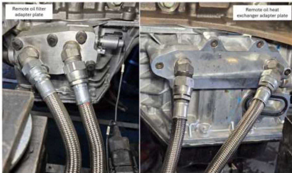
Figure A4.6 Remote oil filter and oil heat exchanger adapter plates example Drawing also available at TMC Website
