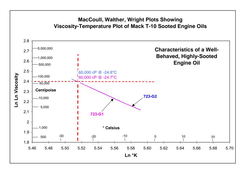
Another view of Oil 723-G run in duplicate showing the simple viscosity-temperature curve and Gelation Index. Repeatability is very good.
