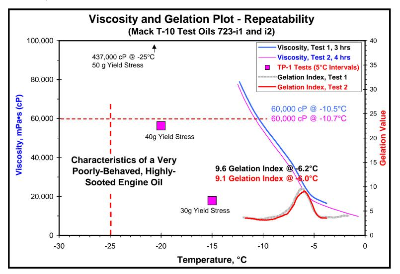
Recording the data continuously from +20°C to -25°C shows that further data can be collected if desired. In the case of Oil 723-E, the oil has a well behaved appearance from +20° to -12°C at which point the oil deteriorates into poor flow behavior.
