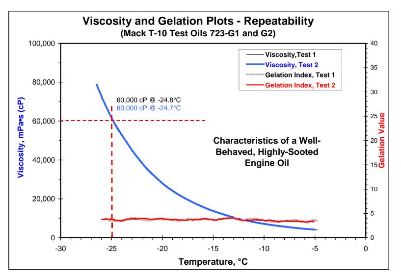
Three TP-1 values obtained at 5°C intervals are added to the information. Agreement of the two instruments is good with well-behaved oil.
