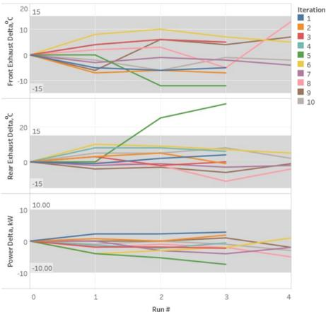
Figure A10.1: Mack T-8E uncontrolled parameter delta from reference test for subsequent candidate tests run in the same stand/engine combination.
