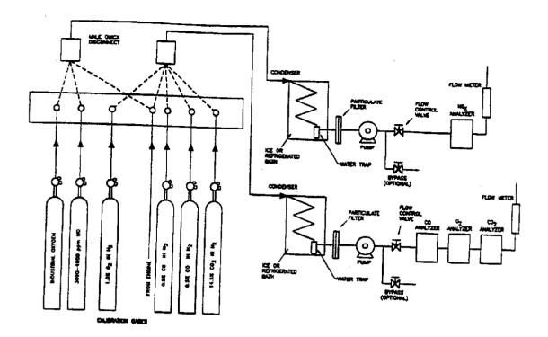
Fig. 8. Exhaust Gas Analysis System
