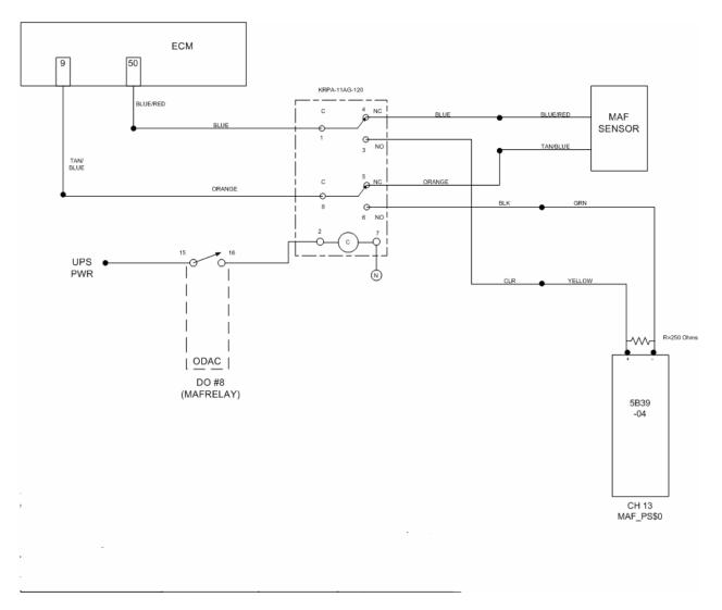
FIG. A3.14 Mass Air Flow Sensor Modifications
