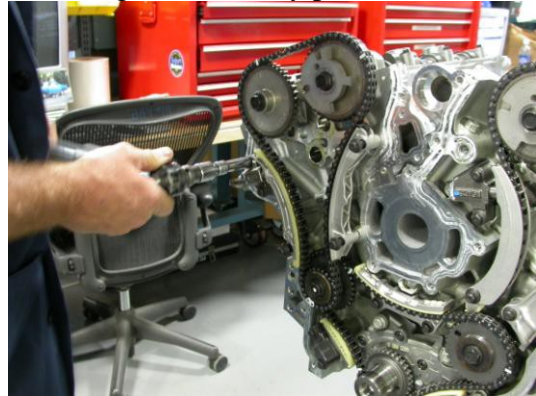
Torque tensioner and chain guides to 23 +/- 3Nm.
