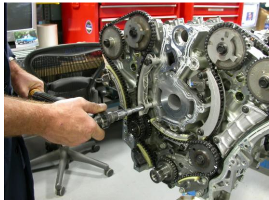
Torque tensioner and chain guides to 23 +/- 3Nm.
