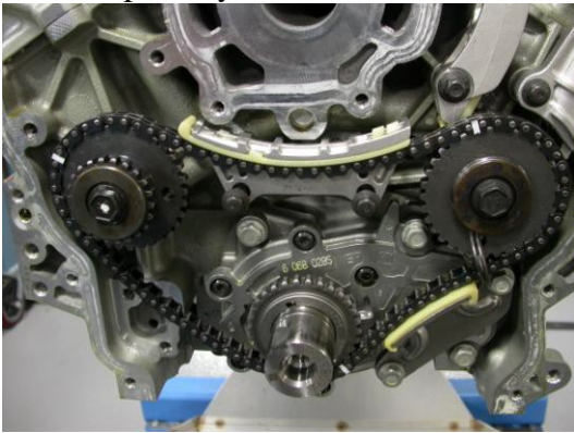
Install primary chain guides.
