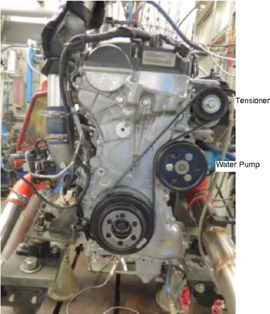
FIG. 7 Water Pump Drive Arrangement
