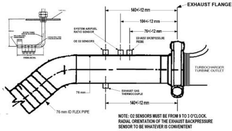
Figure A9.8: Exhaust Measurements and Instrumentation
