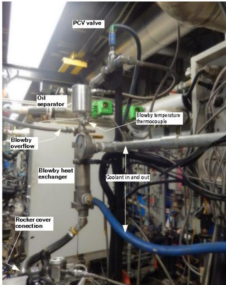
Fig. 11 Crankcase Ventilation System
