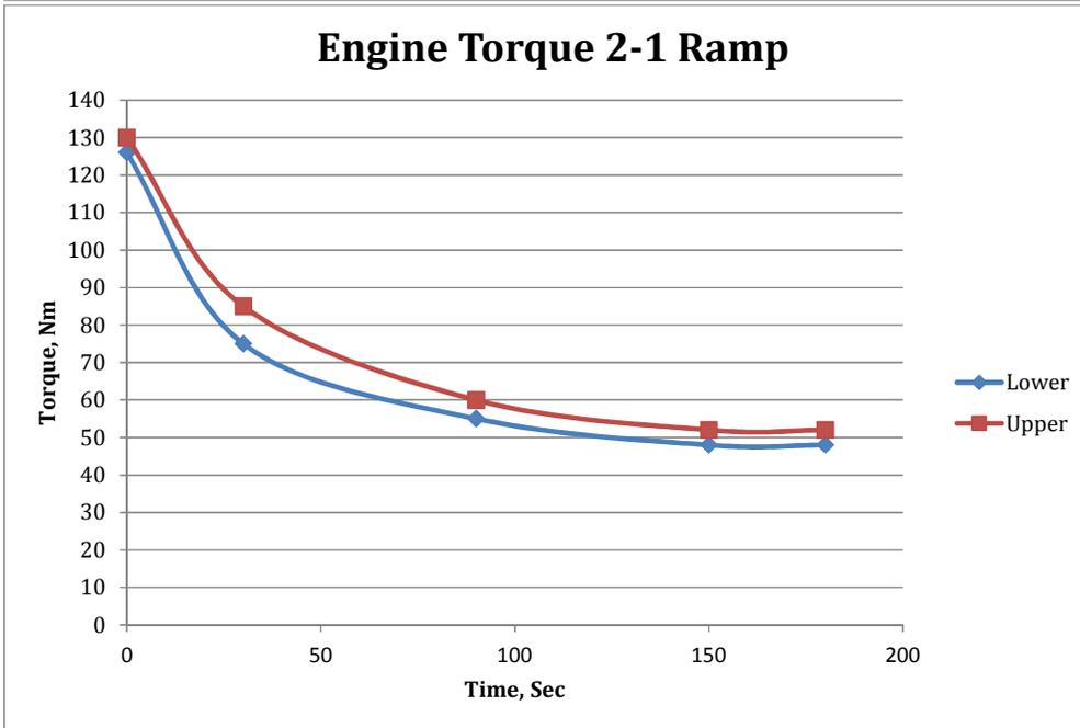
Typical Torque and temperature ramps
