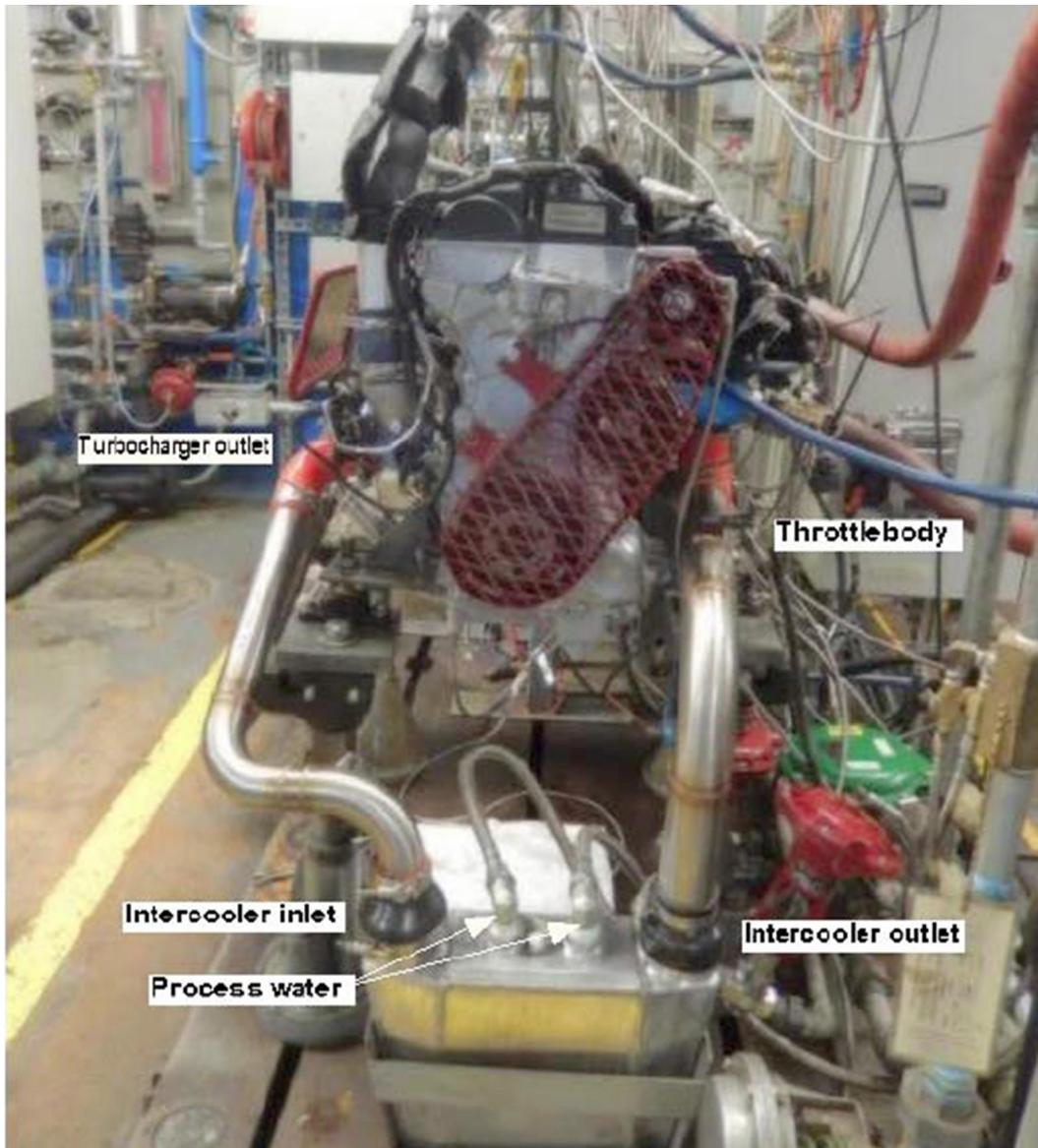
Figure 12, Typical Intercooler Installation
