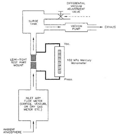
NOTE 1—The inlet flow meter must calibrate to within 5% of the standard (pre-calibrated) orifices at the pressure differentials stamped on the orifices.
