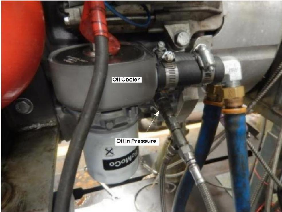
Figure A9.15 Oil cooler showing oil gallery pressure location
