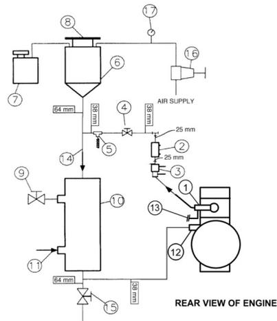
NOTE 1—Observe temperature sensor locations in thermostat housing and at water pump inlet.
