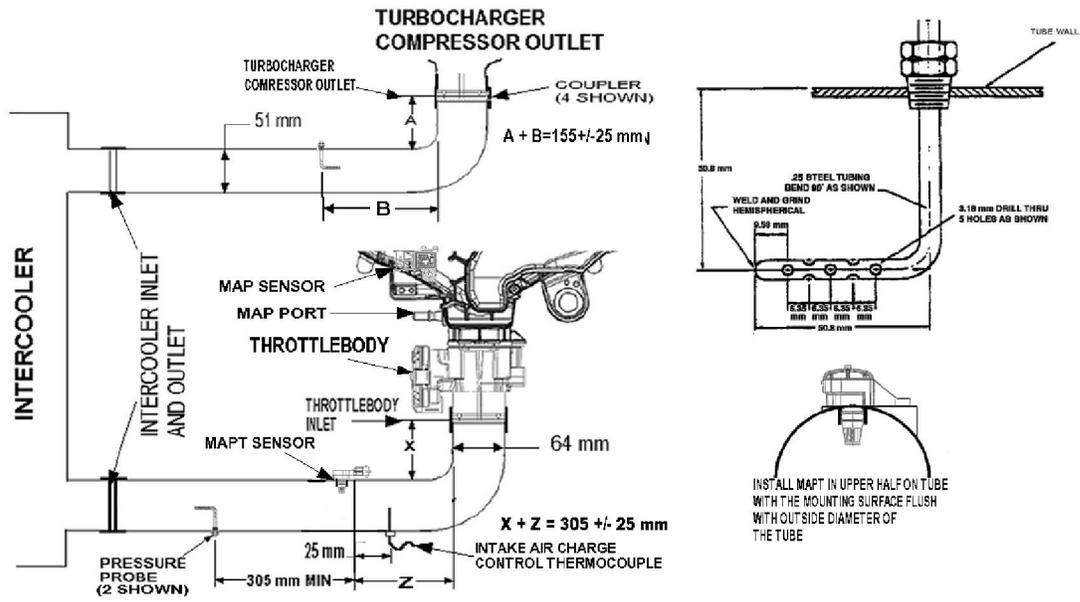
Figure A9.13: Intercooler Tubing Measurements and Instrumentation
