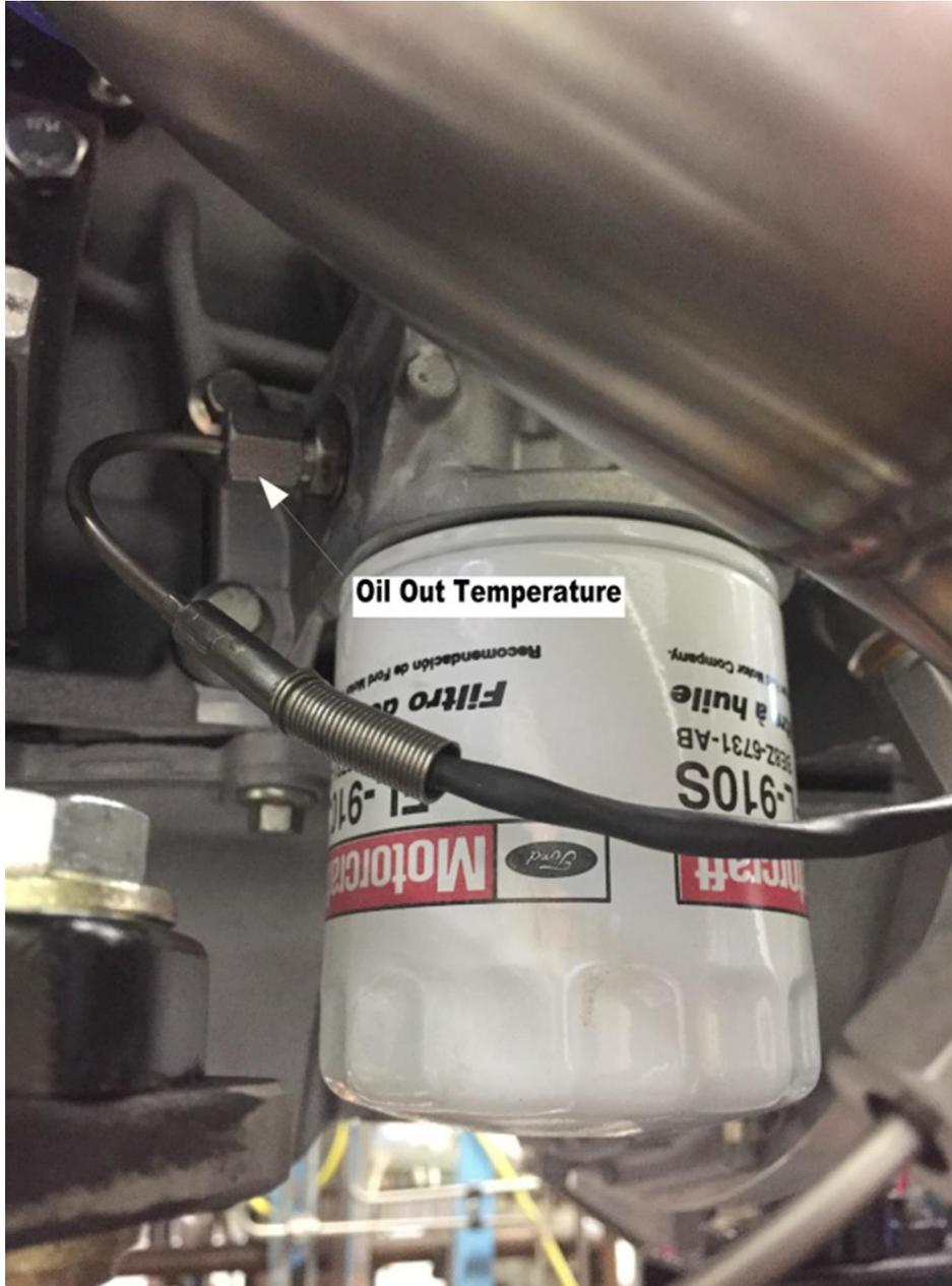
Fig.A 9.3 Oil cooler showing temp measurement locations
