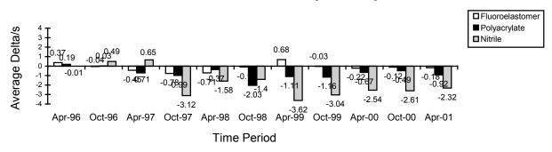
Percent volume industry mean delta/s bar charts for each elastomer material are shown below by report period. Nitrile materials were significantly mild of target. Fluoroelastomer was on or near target and polyacrylate materials trended slightly mild this period. Both labs experienced mild results with the nitrile elastomer, some as high as 13 standard deviations from target.
